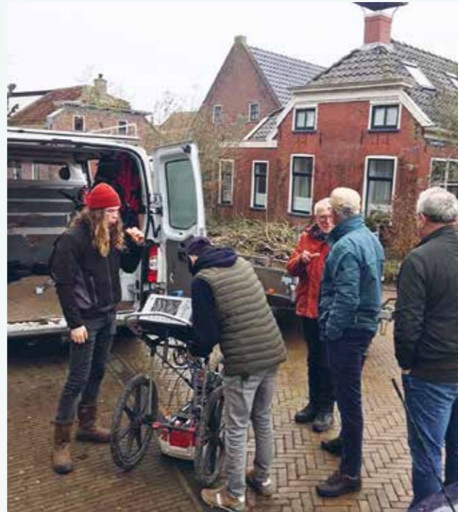
The ground radar of Medusa Explorations is mounted on the chassis of a pram, so that residents' gardens can also be measured.
