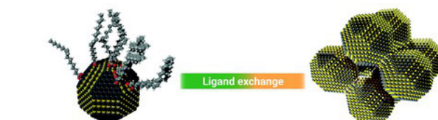
Colloidal quantum dots with truncated cube shape and their original ligands (organic molecules) assembling into an ordered superlattice after the ligand exchange. | Illustration Jacopo Pinna
