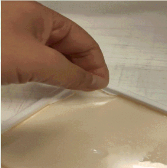
ASSET is a soft, stretchable polymer for wearable electronics | Photo Xiaohong Lan, University of Groningen
